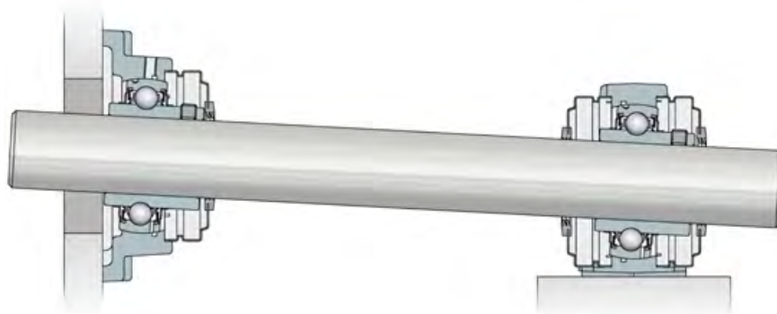
Reduced sealing effect and high wear due to excessive misalignment
