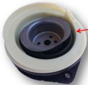
SNR suspension bearing and insulator
