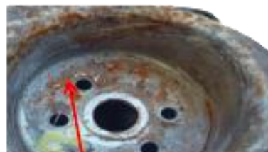
Corrosion caused by movement of the spring
