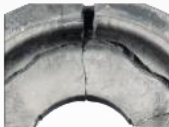
Defective shock absorber bearing:
