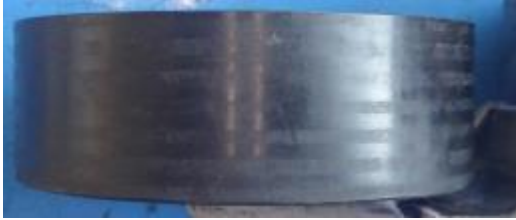
Marks on the pulley
