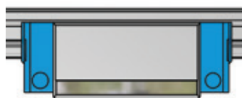
Overhead installation, rotation by 180° y - 180°
