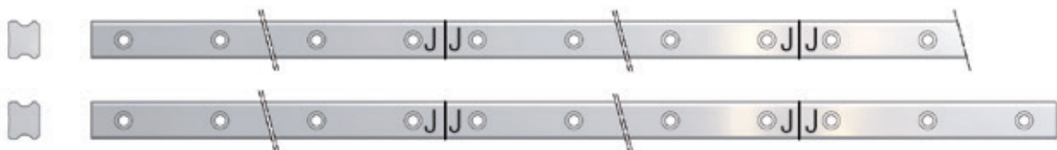
Figure 3.6 Marking of jointed rails
