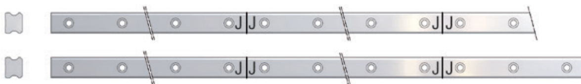
Figure 3.6 Marking of jointed rails
