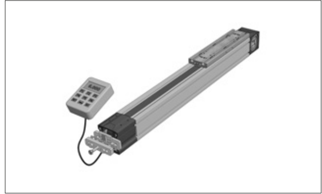
Figure 1.9 Measuring device for the toothed belt tension
