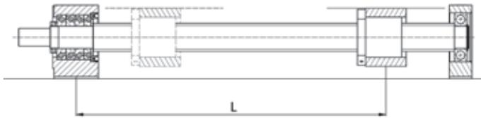
Figure 1.15 Bearing arrangement fixed - supported
