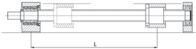
Figure 2.15 Bearing arrangement fixed - supported
