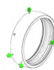
Figure 1 G2 system: Outer ring with four lubrication holes in two planes
