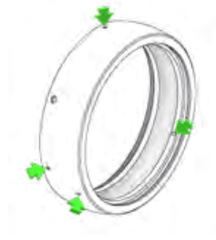
Figure 3 G2 system: outer ring with four lubrication holes in two planes.
