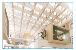
The building will also feature a shed roof, an effective architectural solution for maximising natural light and ventilation, while offering a distinctive and functional design. The roof will be made up of a number of sloping solid and hollow roof surfaces, arranged in sequence. A steep glass slope will face north to avoid direct sunlight but provide constant, high-quality light, while a softer solid slope will face south to avoid excessive heat.
