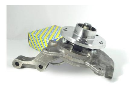
**The ASB3**<sup>®</sup> **load sensor bearing :** this is the last generation of wheel bearing, the outer ring is equipped with gauges. The electronics condition the electrical signals and an algorithm transforms them into loads that are continuously analyzed by the wheel.
